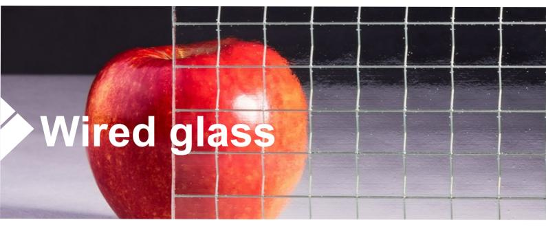
Wired glass is a type of glass with steel that is embedded in it at the production stage. The sunken metal mesh of square mesh is dense enough to hold large shards of glass in case it breaks. The steel prevents the pieces from falling out.
