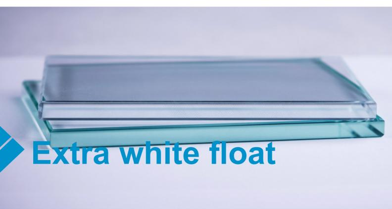
Extra white float is completely discolored glass, obtained by reducing the content of iron oxides in molten glass.
